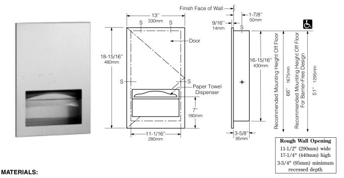
Cabinet — 18-8 S, type-304, heavy-gauge stainless steel. All-welded construction. Exposed surfaces have satin finish.
