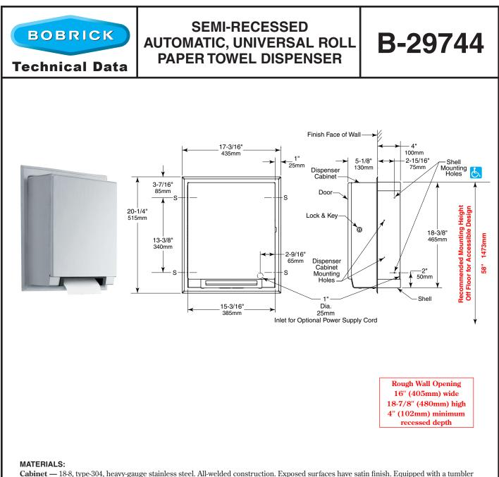
**Cabinet** — 18-8, type-304, heavy-gauge stainless steel. All-welded construction. Exposed surfaces have satin finish. Equipped with a tumbler lock keyed like other Bobrick washroom accessories.
