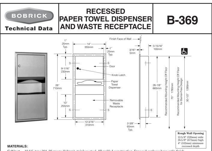
Cabinet — 18-8 S, type-304, 22-gauge (0.8mm) stainless steel. All-welded construction. Exposed surfaces have satin finish.
