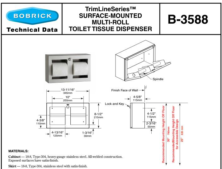
**Door** — 18-8, Type-304, 20-gauge (0.9mm) stainless steel with satin-finish. Secured to cabinet with two rivets. Equipped with a tumbler lock keyed like other Bobrick washroom accessories.
